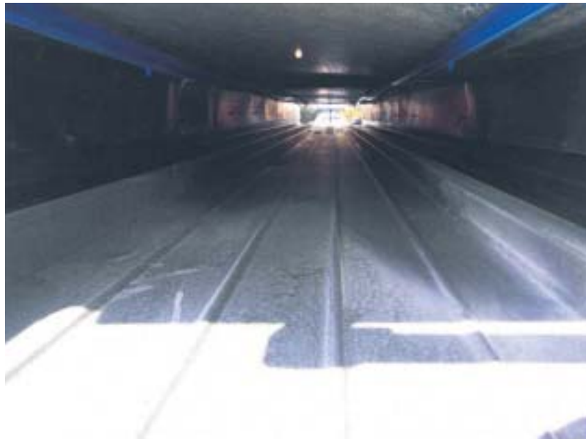
View of the interior part of the sample with the network of spraying nozzles.
