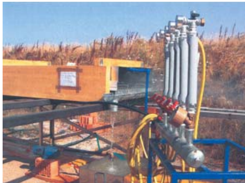
Group of flowmeters.
