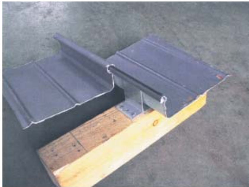
Photograph of the sample subjected to the test: Detail of the connection between the panels and panels- support.
